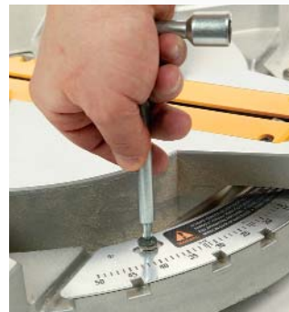
Miter adjustments made easy. Adjusting the miter scale requires loosening only a few screws and sliding the scale/detent plate to the right or left.
