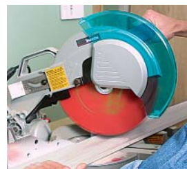
Makita's blade guard is designed not to get caught up on the fence.
