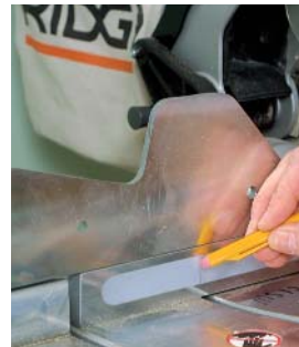
Ridgid's saw comes with an erasable marking strip along the fence.
