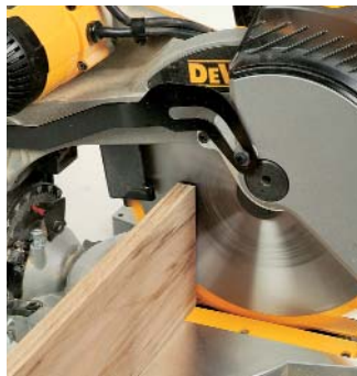
Designed for wide boards. The blade housing on this saw allows 6½-in. boards to be cut standing up against the fence.
