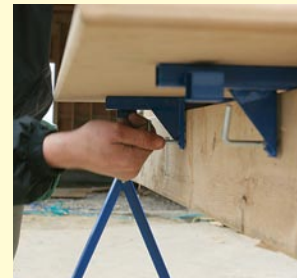
U-channel secures the saw table. Bolted to the underside of the saw table, the U-channel clamps onto the 2x rail.
