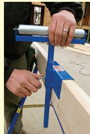
Work supports mount on the rail. The support roller's height is adjusted by loosening a screw clamp. The saw table and work supports can be located anywhere along the 2x rail.
