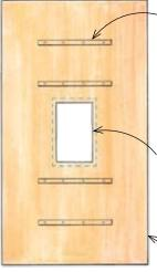
Poplar battens (¾ in. by 1¼ in.) that reinforce the top are glued and screwed to the underside. They're cut and positioned to fit tightly inside the assembled box.
