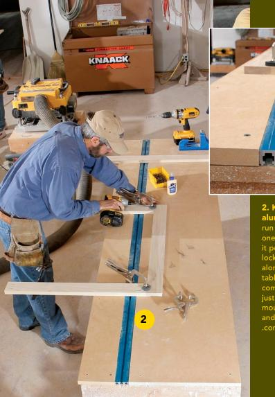
2. Klamp Trak aluminum channels run the full length of one table. This makes it possible to position locking clamps anywhere along the length of the table. The Klamp Trak comes in 34-in. lengths, is just under ¾ in. thick, and mounts using 1/4-20 nuts and bolts (www.kregtools .com; \$45 per track).
