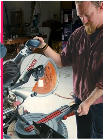
The up-front bevel and miter controls are comfortable to operate, and the tables are smooth enough to be repositioned with one hand still on the main handle. When you are cutting trim, this can equate to hundreds of fewer movements in a workday, saving time and energy.
