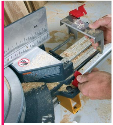
The slide-out extension wings on each end of the cutting table operate smoothly and are in perfect alignment with the table. They have no true equivalent in any other saw I tested.
