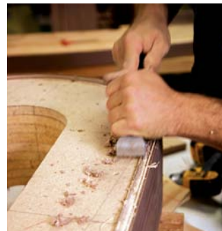
Clean up the edges. When the glue is dry, use a scraper to remove dried glue from the riser's top edge. Even it up with a router and flush-trim bit, using the top of the form as a bearing surface.
