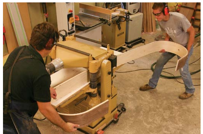
Plane it straight. Remove the riser from the form, and turn it over so that the clean edge rides on the planer bed. Carefully feed the riser through the planer, taking light passes until the riser measures its correct width.
