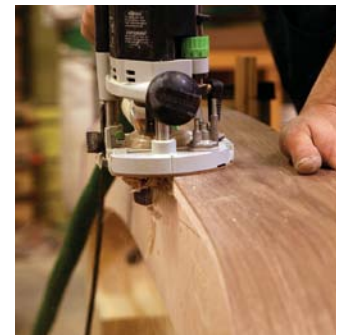
Clean up the edges. When the glue is dry, use a scraper to remove dried glue from the riser's top edge. Even it up with a router and flush-trim bit, using the top of the form as a bearing surface.
