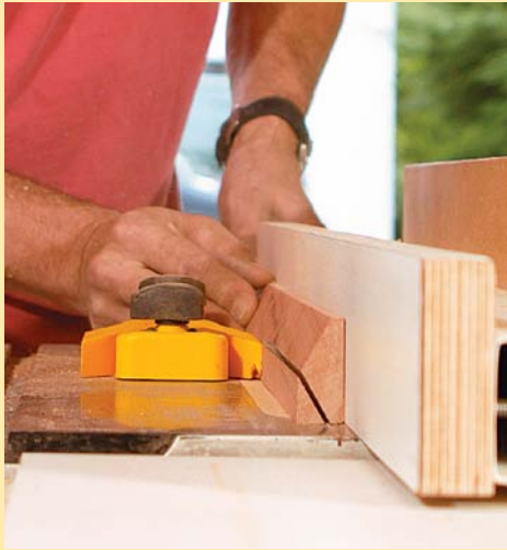
Rip first. After milling lengths of 2-in. by 3/4-in. stock, set the tablesaw to 33° and rip a bevel on both sides of the top.
