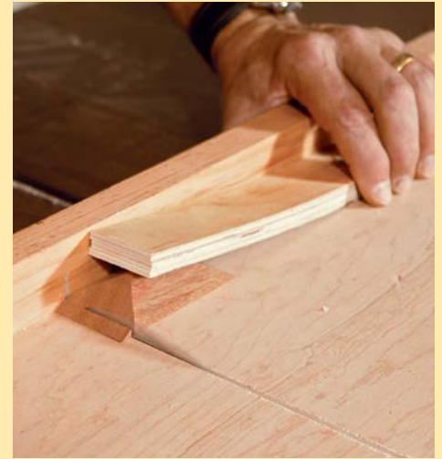
The last cut is a small one. To make the final cut that squares the beveled ends, stack three 1 1/2-in.-wide strips of 1/4-in. plywood and screw them at one end to the sled. The free end is loose enough to act as a spring clamp for holding the small pieces securely as they are trimmed.
