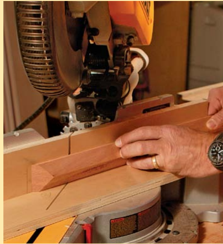
Crosscut next. Moving to the miter saw, make a 59° cut at the end of the stock, advance the piece to a pencil line on the fence, and cut off the pyramid. The pencil line is safer than a hard stop, which would trap the offcut piece where it could be caught and thrown by the spinning blade.
