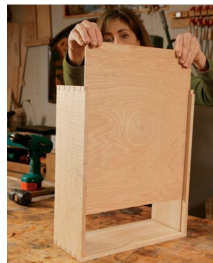
Bottom slides in last. After the glue had dried and the drawer assembly was square and flat, the author slid the plywood bottom into its groove and fastened it with small screws to the underside of the back.
