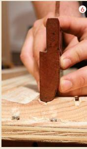
**Rounds cut hollows.** With the inner groove as a guide, use the round plane to cut the dip on each side of the center rib.
