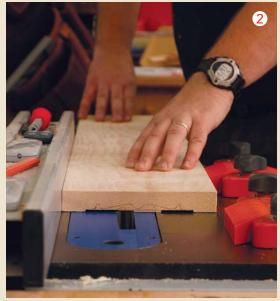
**Remove the waste fast.** After setting up a  $\frac{3}{4}$ -in.wide dado stack, raise the blades to the correct height, and remove the excess stock in several passes, resetting the fence position at each pass.
