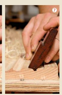
**Hollows cut rounds.** Working from the outer groove, create the rounded portion of the profile with the hollow plane.
