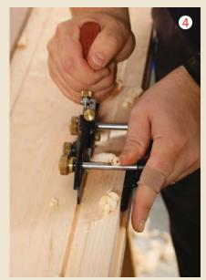
**Define the outer edge.** With the blade set to the required depth and the fence to the correct width, run a narrow plow plane along both edges.
