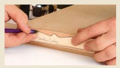
**Plan stock removal.** Once the profile has been traced onto card stock, cut out the silhouette, and trace it onto the trim stock. It's an easy way to see where the most stock can be removed with power tools and where hand planes are most valuable.
