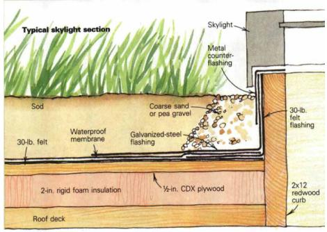
with big gobs of silicone caulk covering both the brackets and the screws. Finally, we place a narrow band of coarse sand or pea gravel along the edge of the 2x4 and around skylights and chimneys to promote quick runoff.
