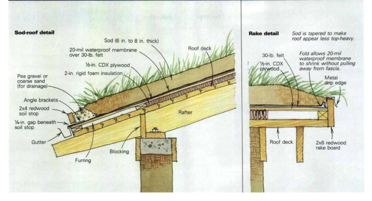
Roof-top anatomy—My state-of-the-art sod roof consists of (from bottom to top) the rafters and decking, 2-in. rigid-foam panels, 3%-in. or ½-in. CDX plywood, a layer of 30-lb. felt, a 20-mil or thicker waterproof membrane, and 6-in. to 8-in. of soil (drawings above). I substitute furring strips for the insulation on the overhangs. A narrow band of gravel or sand promotes drainage along the eaves and around chimneys and skylights.
