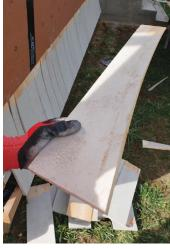
A FAIR CURVE Although typically not thought of as a tool for cutting curves, as long as the flare is relatively gentle, a portable circular saw is an ideal tool for making a quick, smooth cut along the marked line.
